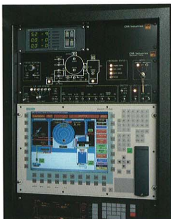
Ergonomically designed modules provide step-by-step control of deposition process.
